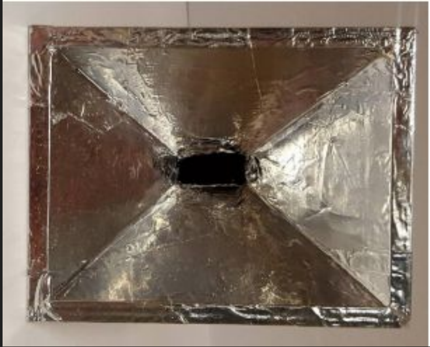
X-band, 15dBi standard gain horn dimensions
